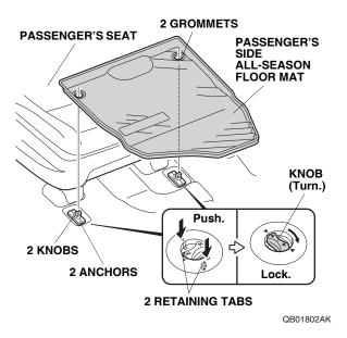
4. Place the grommets in the second row all-season floor mat over the anchors. Push the grommets into
